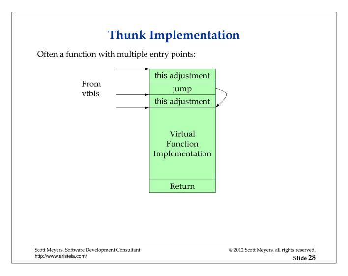
I'm guessing about the jump in the diagram. An alternative would be for one thunk to fall through to the next, with the sum of the offset adjustments calculated to ensure that the proper this value is in place when the function body is entered.
